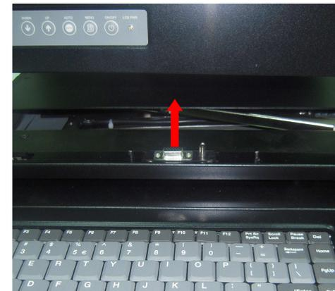
**Step 3.** When installing the new LCD panel take care to correctly align the VGA connector and the locating pins. Fix the panel in place using the 4 screws previously removed.
