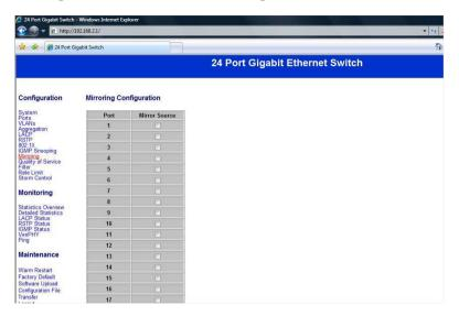
Port Mirroring is for mirror the traffic from Source port to Destination port.
