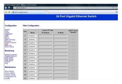
Select the "Port no." which you want to configure the mode to enable/disable filtering IP address.
