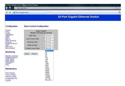
You can set up storm control by configuring the modes.
