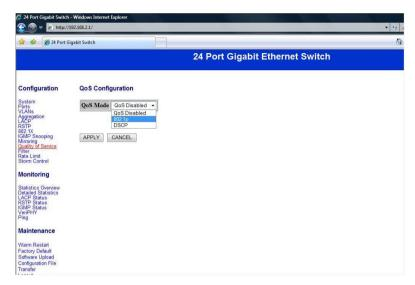
You can enable or disable QoS by clicking the checking box. If you enable QoS, you can select the class of service for each port.
