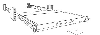
5. Use a screw to connect the blocker to the rear of the console at each side
