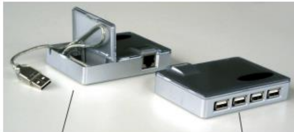
USB Extender Local Unit (Computer side, attach directly to mainboard)
